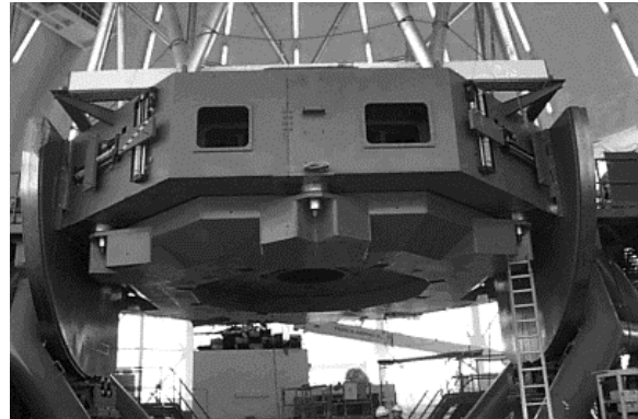
Figure 3. The first primary mirror cell with steel dummy mirror in place in the telescope.
